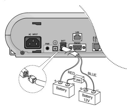
Figure 2.2.7 External Back Up Battery Installation
